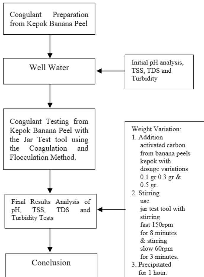
Figure 3.2 Flowchart for Making Coagulant from Kepok Banana Peel
