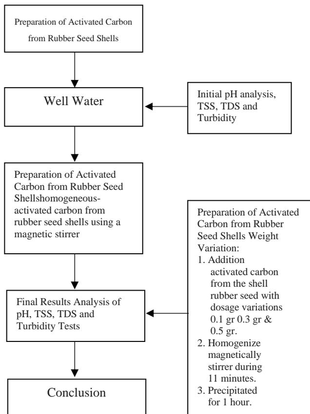
Figure 3.1 Flowchart for Making Activated Carbon from Rubber Seed Shells
