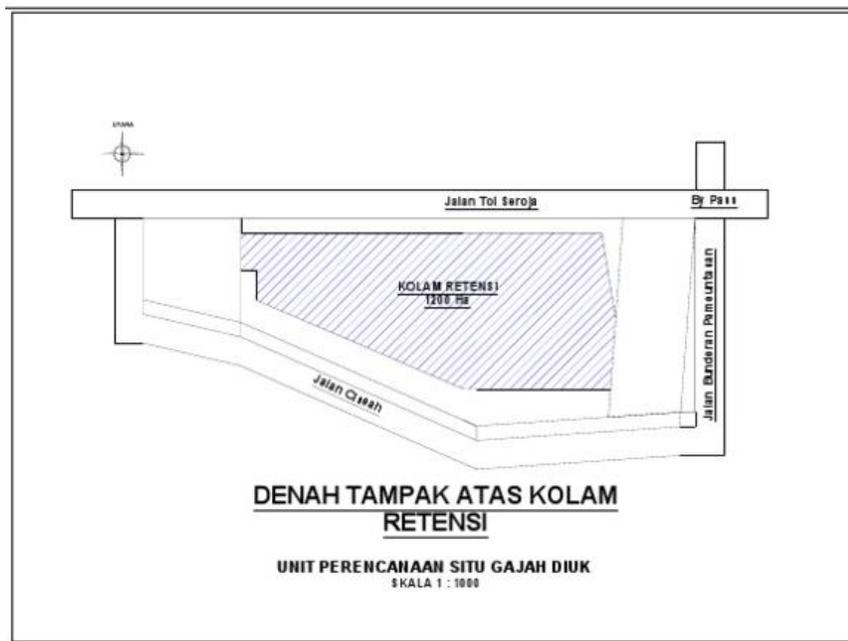
Figure 1. Retention Pool Plan
