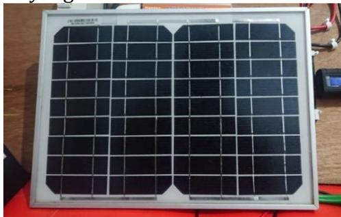
Gambar 1. Panel Surya tipe monokristalin kapasitas daya 20 Wp (Watt peak)
