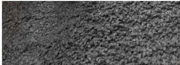
**Gambar 5. Hasil Pencampuran RCC. (Roller Compacted Concrete)**
