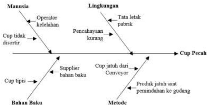
Gambar 4 Diagram *Fishbone* Cup Pecah
