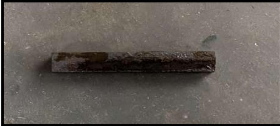
**Gambar 11** Hasil Proses *Quenching* Media Air
