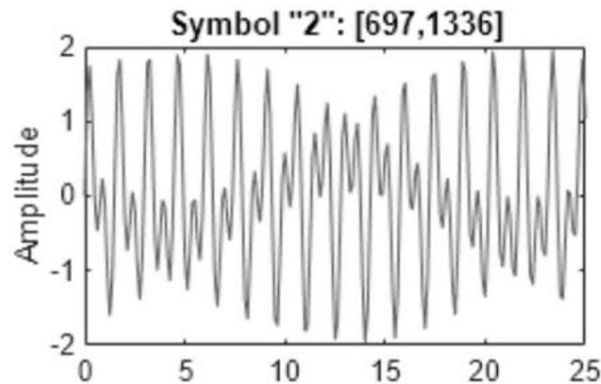
Figure 5. DTMF signal tone 2 or forward movement
