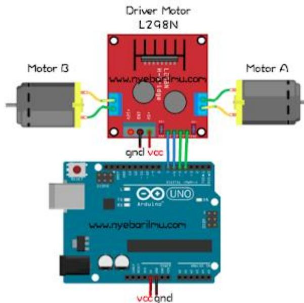
**Figure 3. Arduino Uno and Motor Control Circuit Design**
