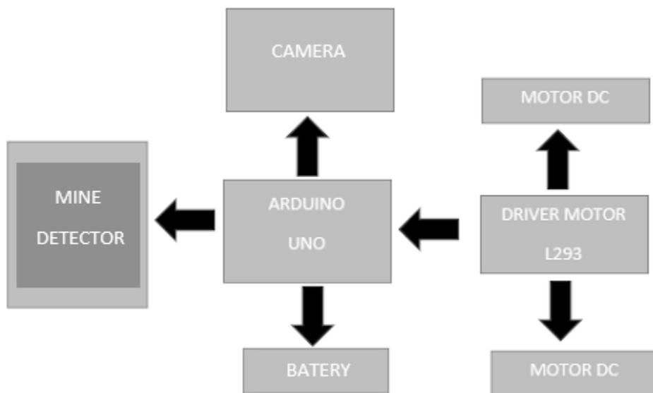
Figure 1. Block diagram of how the robot system works
